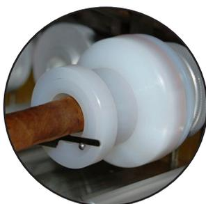
To perform experiments on cigar products, alternative sample holders are required. Cigar holder assemblies are comprised of a filter pad holder, holder assembly, buffer, bobbin, sleeve and holder assembly and can be tailored for specific product sizes. There is a large range of accessories and consumables depending on the size of your Cigar product.
