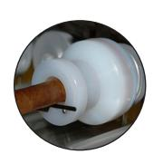
To perform experiments on cigar products, alternative sample holders are required. Cigar holder assemblies are comprised of a filter pad holder, holder assembly, buffer, bobbin, sleeve and holder assembly and can be tailored for specific product sizes. There is a large range of accessories and consumables depending on the size of your Cigar product.
